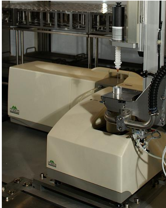
Rheometer, pH and particle size measuring, gel time
