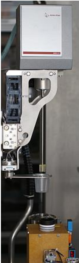
Rheometer, pH and particle size measuring, gel time
